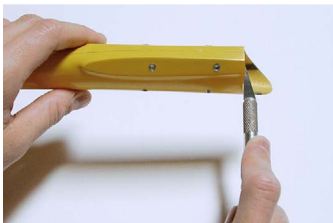
Fig.22: Adjusting the end of the fuselage.
