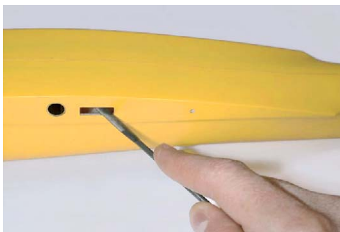
Fig.43: Finish the shape of the hole.
