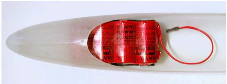
Fig.16: Battery pack in position.
